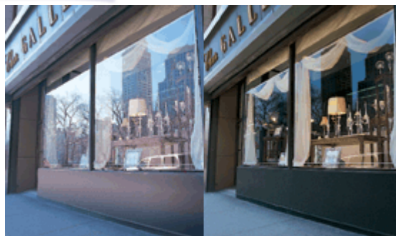
The photo on the left was taken without a polarized lens and the one on the right was taken with a polarized lens. Notice how the polarized lens reduces glare.
